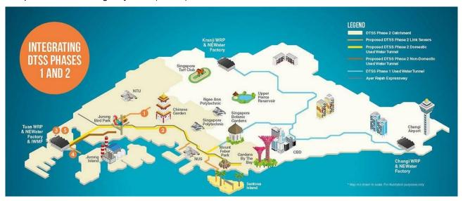
The first batch of deep tunnels and link sewers, amounting to 30km, together with the other phases, is expected to complete by 2025. It will be connected to the Tuas Water Reclamation Plant to transport water into the 3 centralised water reclamation plants, with the aim of increasing water recycling rate.
